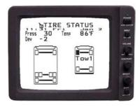
Using the up  $\Delta$  and down  $\overline{V}$  keys will let you scroll through the tires to display pressure, temperature, and pressure deviation readings for each tire.
