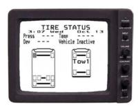
Press the VIEW key on the keypad to switch between standard rear vision screen and "TIRE STATUS" screen. If the "TIRE STATUS" screen is not accessible and the "TIRE SYSTEM DETECTED" message is displayed, your tire monitoring system has not yet been configured. Press <u>RESET</u> and follow the instructions in the "Programming for Tire Sensors" section.
