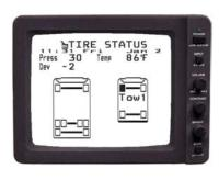
The respective tire icon lines become solid as soon as data from its transmitter is received. When your vehicle is driven over 6 mph, the TripTek® system will begin to receive tire data. After data from all transmitters is received the display will be in a state similar to that shown at left until an alert condition is detected.
