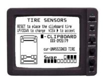
The following procedure will require two people, one to drop the air pressure of a specific tire and the other to track data. Have one person drop the air pressure of a specific tire by approximately 4 PSI to activate the tire sensor. When activated, the sensor will transmit a signal to the TripTek computer. While the pressure is being dropped the transmitted signal will display a filled tire in the SWAP section of the "TIRE SENSORS" screen.
