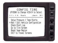
Using the up  $\triangle$  or down  $\overline{\nabla}$  keys move arrow to Add/Edit Vehicle Configuration.
