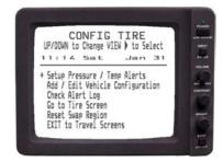
Using the up  $\triangle$  or down  $\overline{\nabla}$  keys move arrow to Setup Pressure/Temp Alerts.
