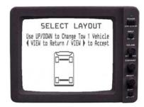
Press the up  $\triangle$  or down  $\nabla$  keys to select vehicle type. Press VIEW  $\blacktriangleright$  to accept.
