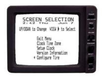
Using the up  $\Delta$  or down  $\nabla$  keys move arrow to Configure Tire.
